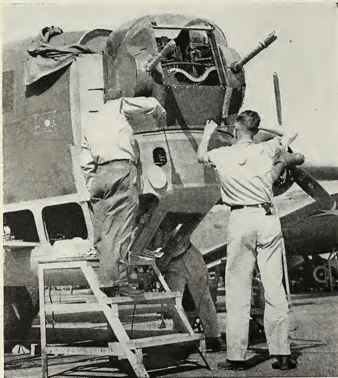
Oklohomo City Air Depot workers fasten the final bolts and screws in mounting a new stinger in the nose of a B-24. The glass front pieces are installed after the turret is tightened in place.
